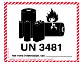
We advise that when shipping these batteries by air, that IATA regulation UN3481 PI966 is followed. This states that the battery must be packed with its associated control gear and the above label must appear on the outer packaging.
