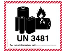
We advise that when shipping these batteries by air, that IATA regulation UN3481 P1966 is followed. This states that the battery must be packed with its associated control gear and the above label must appear on the outer packaging.
