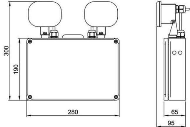
The CT6S/6W/NM3 is a simple solution to your emergency lighting applications. The only connection required is a permanent Live, Neutral and Earth.
